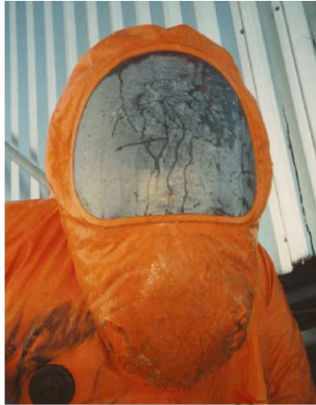
Figure 5. Misting of visor was a problem with Suit B
